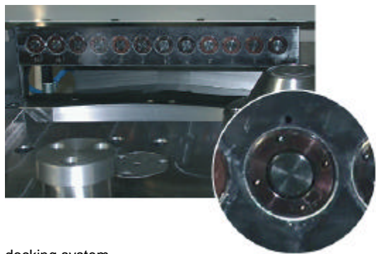
docking system to connect tools in large presses
